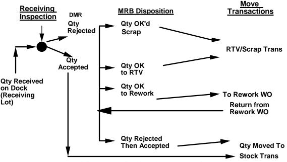
**Receiving Inspection & Rejected Material Flow**
